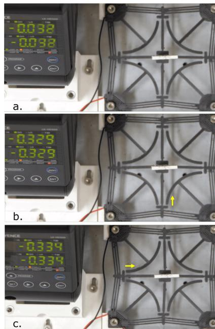
**Fig. 19** Experimental setup of the XY positioning system. The numbers on the dials of the Keyence sensor show the displacement in centimetres. The top image (a.) represents the initial state and the middle (b.) and bottom (c.) images show the amount of displacement in the direction of the arrows in response to an actuation.
