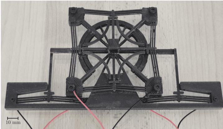
**Fig. 20** 3D printed monolithic XYZ $\theta$  positioning system
