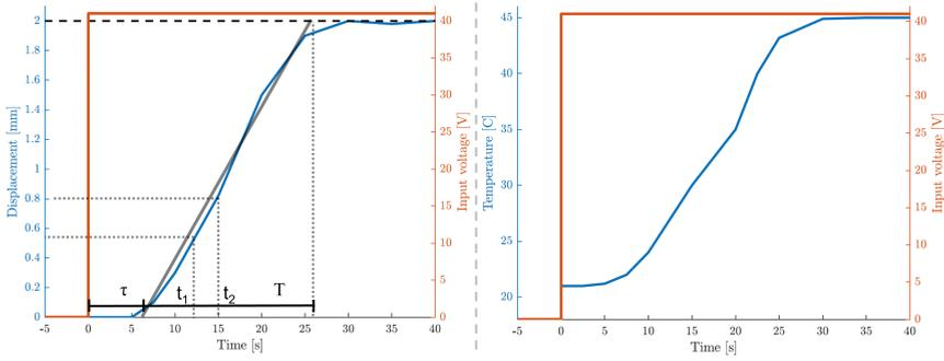
**Fig. 22** On the left, the step response of the system representing the displacement of the actuator as a function of time following power-up. On the right, the intermediate response of the system where the temperature evolution after power up is represented. The delay is present during the temperature rise of the system.
