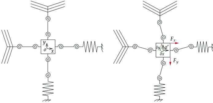
**Fig. 4** Illustration of the working principle of the compliant mechanism for linear motions on two axes. Deflections and compressions are represented by spiral and linear springs.
