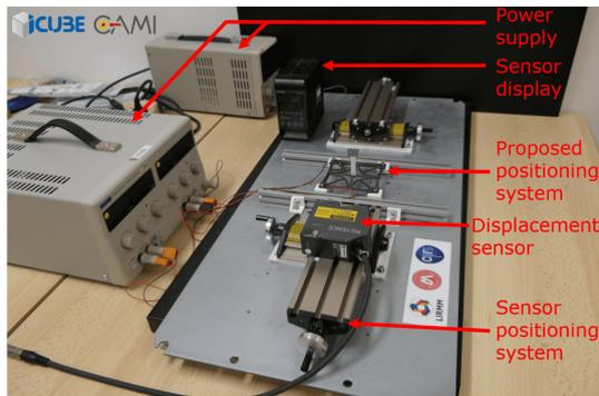
**Fig. 18** Experimental setup of the XY positioning system.
