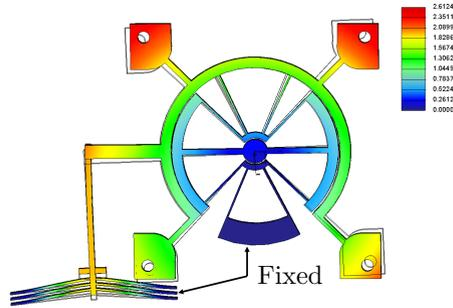
**Fig. 14** Finite element simulation result of the rotational guiding system (displacement in mm).
