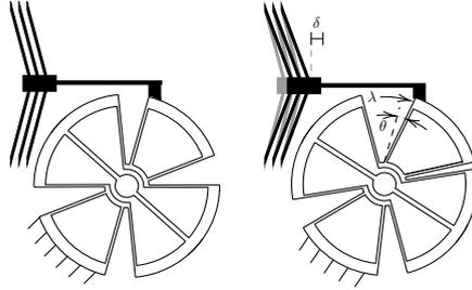
**Fig. 7** Schematic of a two-blade RCC pivot and its integration into a half-pin (symmetrical on both sides of the axis)
