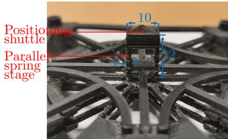
**Fig. 8** 3D-printed monolithic Z linear guiding (unit: mm).
