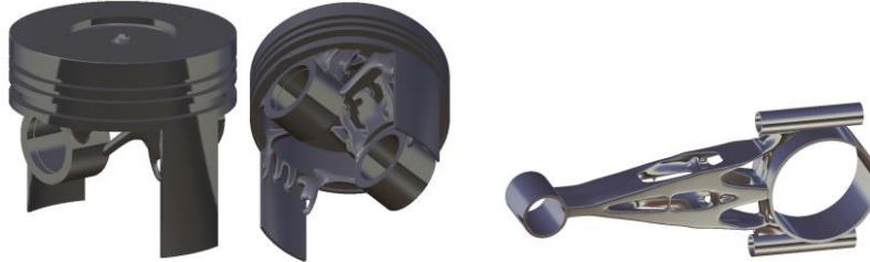
Fig. 22. Redesign of the piston on the left and the connecting rod on the right.
