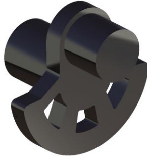
Fig. 21. Redesign of the crankshaft after optimisation for path 1 (colour figure online)
