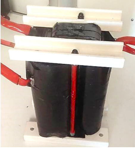
Figure 5: MFT with the common-mode insulation distances for the HV coil, the total weight is 14kg.
