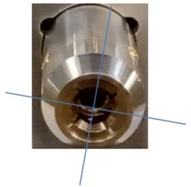
Figure 9: Rotation of the electron gun
