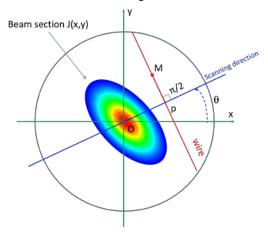
Figure 2: Geometry of the scanning apparatus
