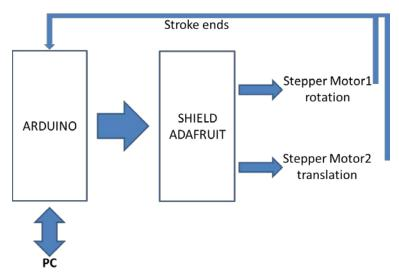
Figure 4: Synoptic scheme of the motor driving
