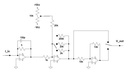
Figure 5: Electronic scheme of the current amplifier
