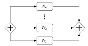
Figure 3. Parallel execution of workflows (AND).
