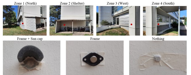
Fig. 2. Top: Location of the four zones (red dot). Bottom : iButtons set-ups
