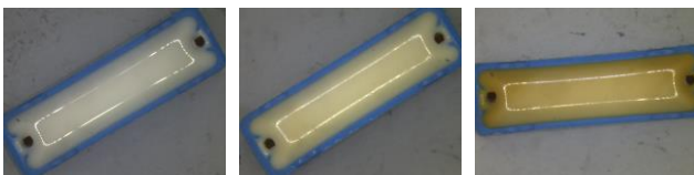
Fig. 17: Capacitor 1 insulating material after steps at temperature, from left to right, 80°C, 100°C and 120 °C.
