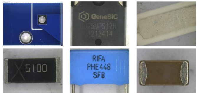
Fig. 14: Tested components before immersion, from top left to bottom right: PCB, diode, resistor 1, resistor 2, capacitor 1, capacitor 2.
