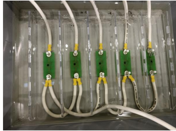
Fig. 9: Test set-up of the PCB samples, after a batch of tests (black spots where breakdown happened)
