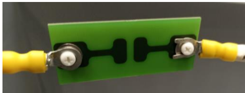
Fig. 8: Sample PCB with 3 mm gap and 70 \mu\text{m} thick traces
