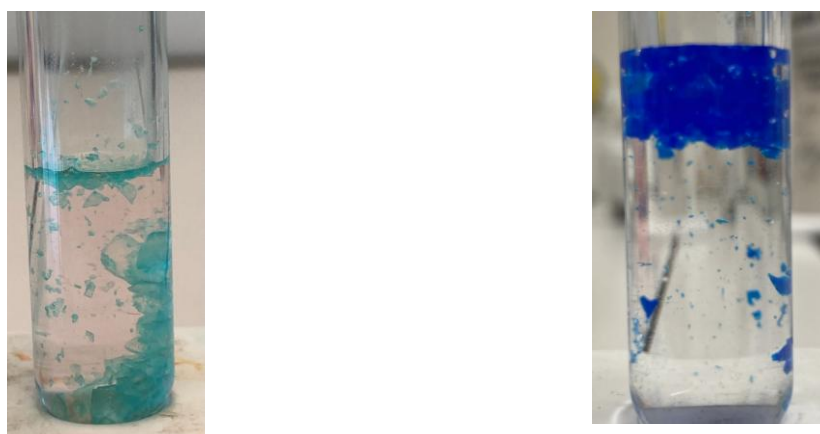
Figure 4: Snapshot after extraction of Co(II) of ionogel [THN][Br] (left) and of the ionogel [THN][Br] treated by NaDca (right). [\text{Co}(\text{II})] = 1.5 \times 10^{-2} \text{ mol.L}^{-1} ; V_{\text{aq}} = 2 \text{ mL} , m_{\text{ionogel}} = 0.300 \text{ g}
