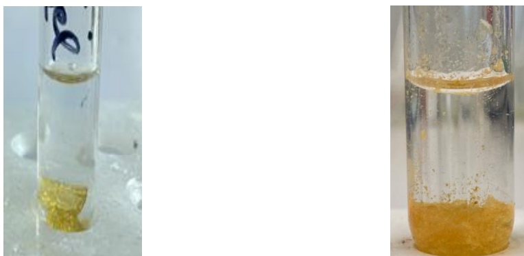
Figure 6. Snapshot of ionogel after extraction of \text{AuCl}_4^- (left) and \text{PtCl}_6^{2-} (right) from [\text{THN}][\text{Br}] ionogel. [\text{Au(III)} (\text{Pt(IV)})] = 1.5 \cdot 10^{-3} \text{ mol.L}^{-1} ; V_{\text{aq}} = 2\text{mL} , m_{\text{ionogel}} = 0.300 \text{ g}
