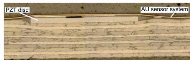
Figure 1: Fiber misalignment under a cobonded sensor [7]
