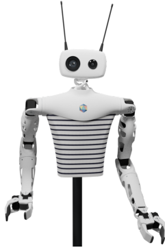
Figure 3: Reachy's Full kit picture: 3D printed MJF Painted - Flexible PU molded - Aluminium Construction; 670x1800x200mm with arms outstretched; 180 W of Max Power consumption and 6.2 kg of weight.
