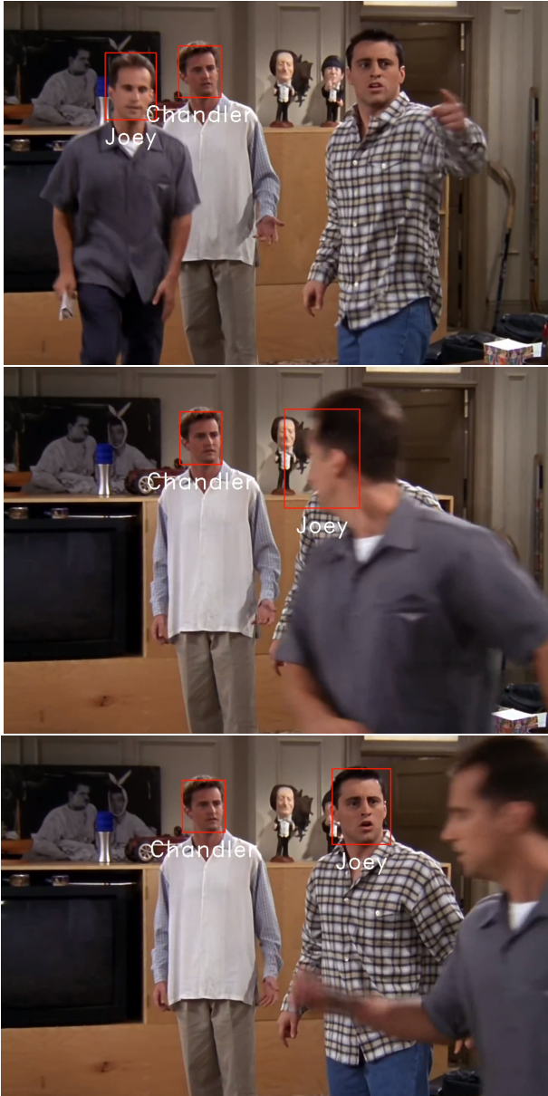
Figure 7: Case where one character occludes another one. We present 3 frames of the same shot ordered by time from top to bottom. Initially, the two characters (the man with grey shirt and Joey) are correctly tracked. But then, the occlusion of Joey by the other man, combined with the fact that the man moves too fast to be correctly detected by the head detector, leads to a confusion between the two tracklets of both characters. The method keeps only the tracking of the man in grey before the occlusion, and the tracking of Joey after the occlusion. The best face in this mixed tracklet is Joey’s (as it is visible from front and motionless), so after annotation, his name was propagated to the other character.
