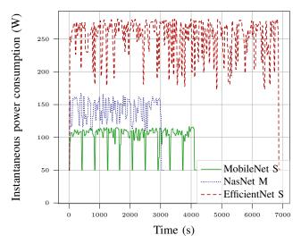
Figure 2: Nvidia A100 power consumption for 3 architectures
