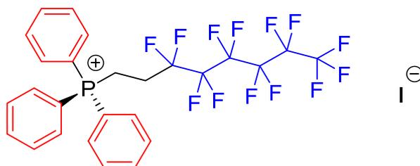
**Scheme 1.** Chemical structure of perfluorooctyltriphenylphosphonium iodide (IL-C8F13).
