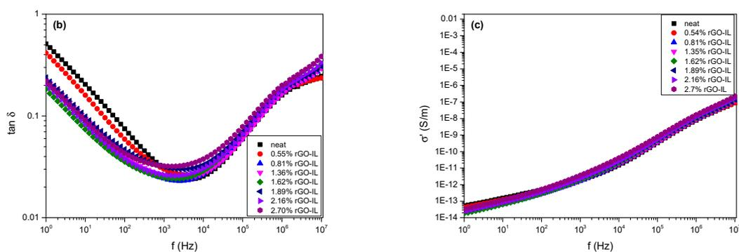
**Figure 15.** Relative dielectric permittivity ( $\epsilon_r'$ ) (a), loss tangent ( $\tan \delta$ ) (b), and AC conductivity ( $\sigma$ ) (c) of P(VDF-CTFE)/rGO-IL composites as a function of frequency at RT with different compositions.
