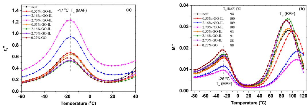
**Figure 13.** Imaginary part of relative permittivity ( $\epsilon_r''$ ) (a) and dielectric modulus ( $M''$ ) (b) as a function of the temperature of neat P(VDF-CTFE) and composites containing GO, GO-IL, and rGO-IL ( $f = 1\text{ kHz}$ , the first heating run). Note that the peak position and intensity from the first heating run is the same as the one from the second heating run).
