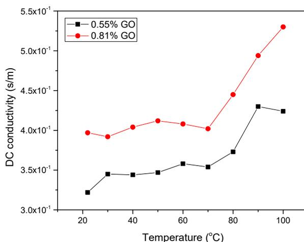
**Figure 14.** Direct current (DC) conductivity as a function of temperature of P(VDF-CTFE)/GO.
