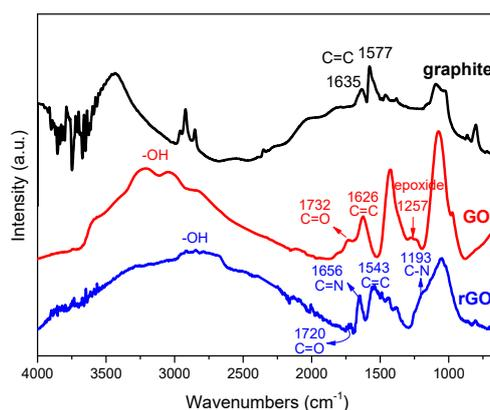
**Figure 3.** Attenuated total reflectance Fourier transform infrared (ATR-FTIR) spectra of graphite, GO, and rGO.
