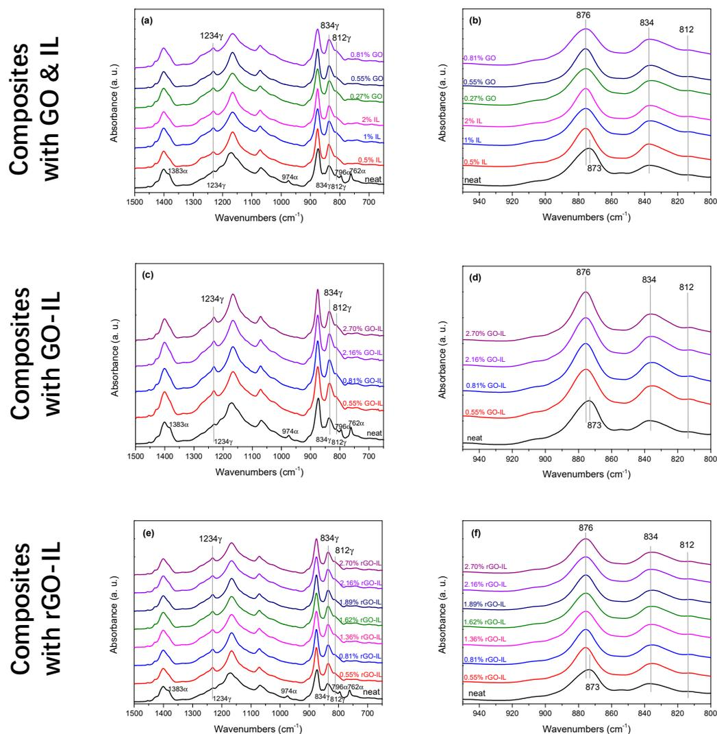
**Figure 12.** ATR FTIR spectra of neat P(VDF-CTFE) and composites with IL, GO (a,b); GO-IL (c,d); and rGO-IL (e,f).
