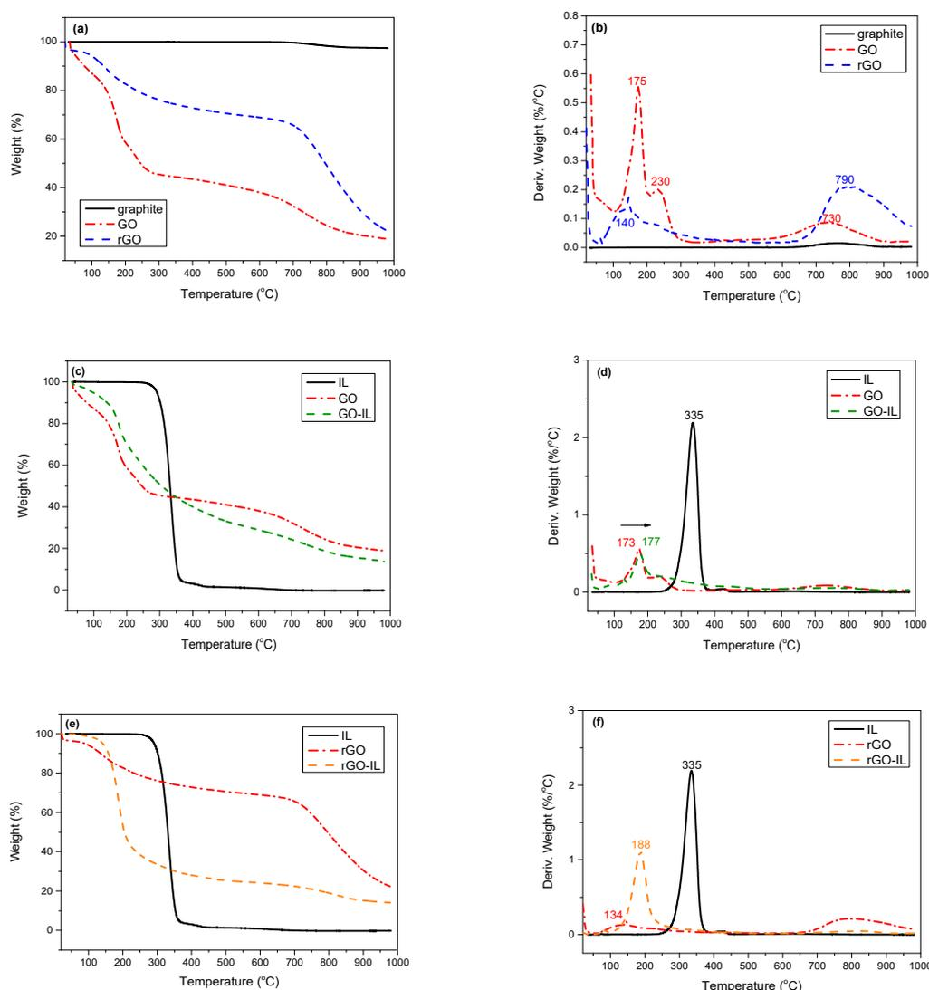
**Figure 1.** Thermogravimetric Analysis (TGA) (a) and derivative thermogravimetry (DTG) (b) thermograms of graphite, graphene oxide (GO), and reductive graphene oxide (rGO); TGA (c) and DTG (d) curves of GO, IL, GO-IL; TGA (e) and DTG (f) curves of rGO, IL, rGO-IL under  $N_2$  atmosphere.
