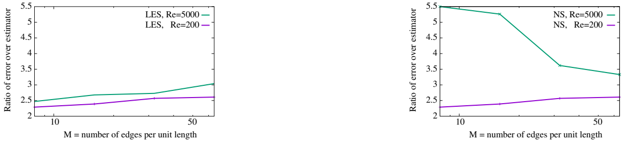
FIGURE 2. Estimation of ratio of errors over estimators with (left) and without (right) LES.
