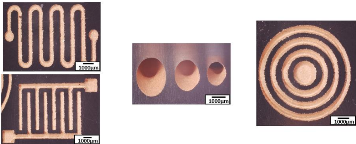
SI2: Optical microscopy images of different metallized patterns on the cube sample.
