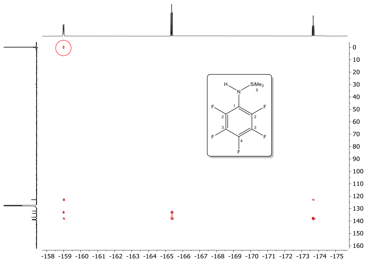
Fig. S17. HMBC ^{19}\text{F} - ^{13}\text{C} NMR (benzene- d 6 , 470.55/125.78 MHz, 27 °C) of N -(pentafluorophenyl)-trimethylsilylamine (3-H). The circled correlation spot demonstrates ^5J_{\text{C},\text{F}} scalar coupling between o -F atoms and Si(CH 3 ) carbon atoms.
