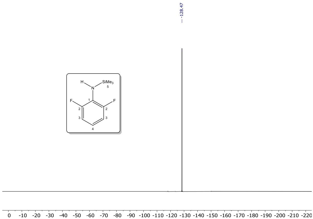
Fig. S11. ^{19}\text{F} NMR spectrum (benzene- d_6 , 282.36 MHz, 25 °C) of N -(2,6-difluorophenyl)-trimethylsilylamine ( 2-H ).
