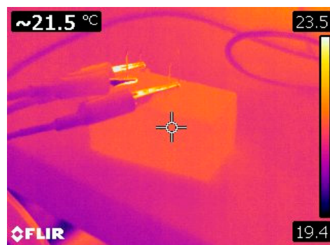
Figure 6. Samples 40 \times 40 \times 80 \text{ cm}^3 with MWCNTs and electric field measurement.
