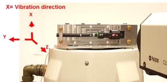
Fig. 12. Lateral excitation (parallel to X-axis)
