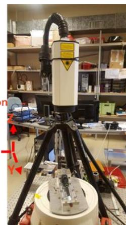
Fig. 13. Vertical excitation (parallel to Z-axis)
