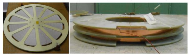
Figure 3 - Left: non-inductive coil for SFCL (Ø690 mm) [10]. Right: Inductive coil for SMES (Ø240 mm) [12].
