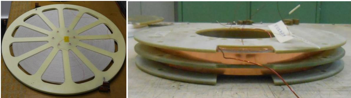
Figure 3 - Left: non-inductive coil for SFCL ( $\phi 690$  mm) [10]. Right: Inductive coil for SMES ( $\phi 240$  mm) [12].
