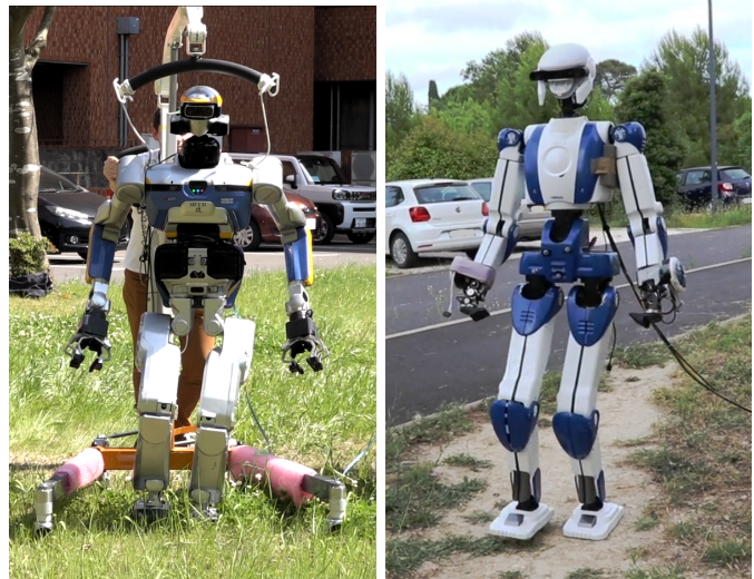
Fig. 1: HRP-2KAI and HRP-4 robots walking outdoors. Experiments with the HRP-4 are done without safety ropes.
