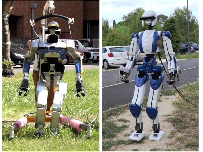
Fig. 1: HRP-2KAI and HRP-4 robots walking outdoors. Experiments with the HRP-4 are done without safety ropes.
