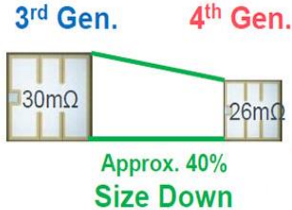
ROHM SiC die size shrinkage leading to high power loss density
