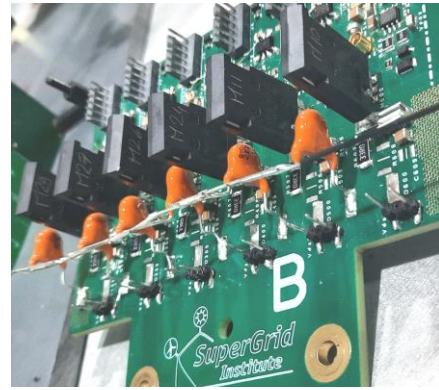
Fig. 7 A photograph of the 10 kV switch with capacitances connected between the drain terminals and the ground. The capacitances emulate the parasitic common mode capacitance introduced by packaging.
