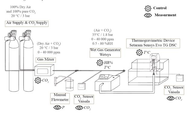
Figure 2: Schematic view of the experimental set-up for carbon dioxide retention measurement
