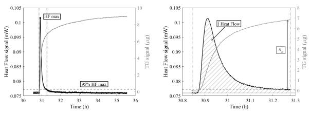
(a) Full heat flow signal for a given  $CO_2$  concentration (b) Extracted heat flow signal between the limits of integration for a given  $CO_2$  concentration
