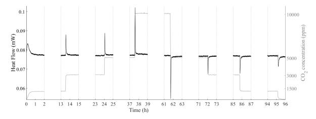
Figure 4: Heat flow signal of the sample exposed to successive levels of  $CO_2$  concentrations: 1500, 3000, 5000, 10000 ppm, at 35°C and 0.5% RH
