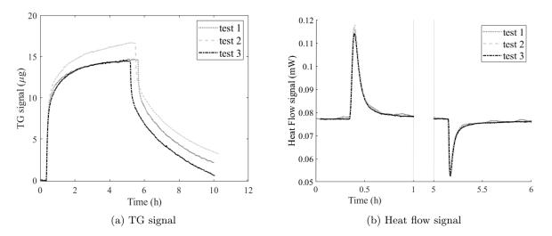
Figure 7: TG (a) and heat flow signals (b) with time of 3 samples exposed to the same conditions (5000 ppm,  $35^{\circ}$ C and 0.5% RH)
