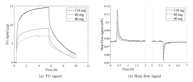
Figure 8: TG (a) and heat flow (a) signals with time of 3 samples with different initial mass exposed to the same conditions (5000 ppm,  $35^{\circ}$ C and 0.5%RH)
