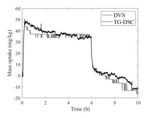
Figure 6: Mass uptake of the samples inside the TG-DSC apparatus (black) and DVS apparatus (grey) when exposed to 5000 ppm, 35°C and 1% RH.
