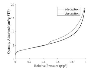
Figure 1: Nitrogen adsorption desorption isotherm at 77 K for 3 g of DAG earth
