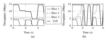
Figure 3. Exemplary resource utilization for three slices. (a) Static resource reservation. (b) Dynamic resource reservation.
