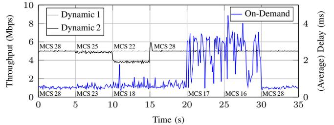
Figure 6. Behavior of dynamic (rate) and on-demand slices (delay) if user channel quality changes. The delay is an average over 100 ms.
