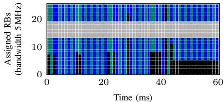
Figure 8. RB allocation for multiple slices: (light gray) fixed slice, (blue and green) two dynamic slices, (black) on-demand slice.
