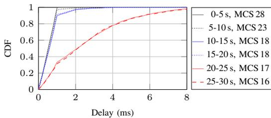
Figure 7. Comparison of scheduling delay for changing user channel qualities.
