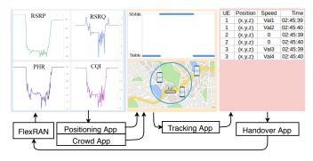
Fig. 3: Sample use case with serial and parallel data flow pipelining. Notice the three layers of the serial part of the chain from left to right: blue, feeding Positioning and Crowd Apps in parallel; yellow feeding the Tracking app; orange, feeding the Handover App.
