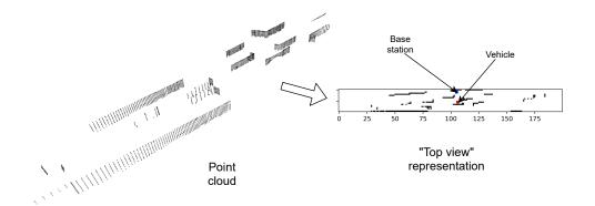
Fig. 1: Preprocessing of the LIDAR point cloud.
