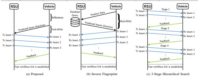
Fig. 8: Timing diagrams of (a) the proposed NN-based beam alignment protocol using LIDAR and position information, (b) the inverse fingerprinting scheme using position information only [23] and (c) a 3-stage hierarchical search [22].
