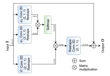
Fig. 3: Block diagram of the non-local attention module.
