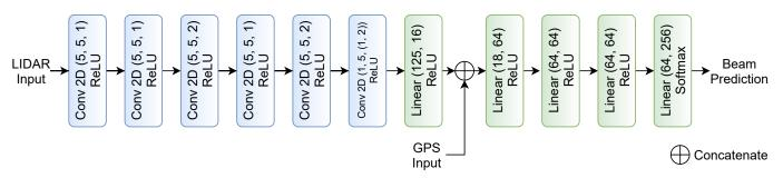
Fig. 2: The proposed CNN model architecture.
