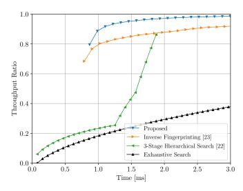
Fig. 9: Throughput ratio versus beam sweeping time. The proposed and the inverse fingerprint schemes curves are obtained evaluating the schemes for different values of K. They introduce a modest overhead to the overall beam training but they are able to perform a more efficient informed search compared to the hierarchical and exhaustive sweeping algorithms.
