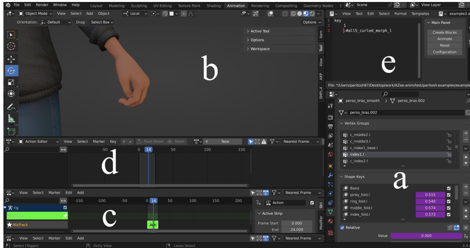
Fig. 6: Blender interface. (a) Shape Key properties (b) 3D Viewport (c) Non-linear Editor (d) Action Editor (e) AZee editor
