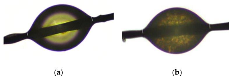
Figure 2. Influence of the annealing treatment on the microbond crystalline state: (a) after fast cooling; (b) with an annealing treatment.
