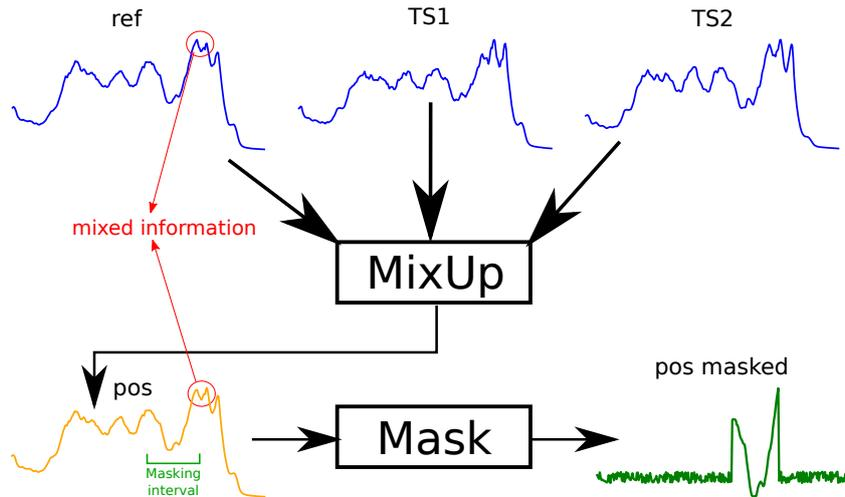
Figure 3: A *pos* (in orange) is built from three time series including the *ref* (in blue). The resulting time series is close to the *ref* except some areas as highlighted in the red circle. A mask is then applied on the mixed up *pos* to generate the final sample (in green), where the unmasked parts are replaced by a Gaussian noise.
