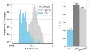
(a) Latency comparison: 100K mes- (b) CPU comparison sages sent at 4K rate (msg/s)
