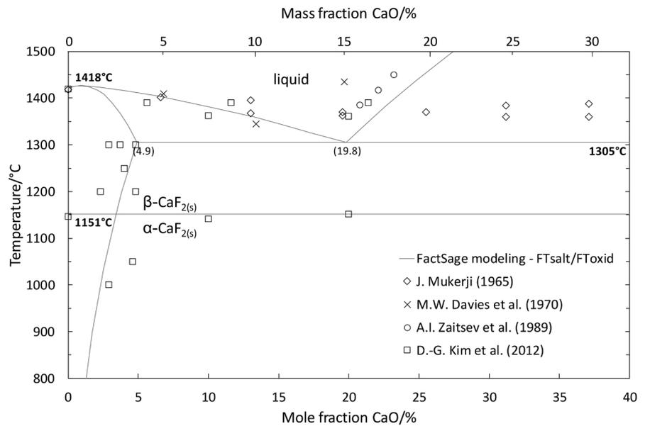
**Figure 6.** Calculated phase diagram of the CaF<sub>2</sub>-CaO system.
