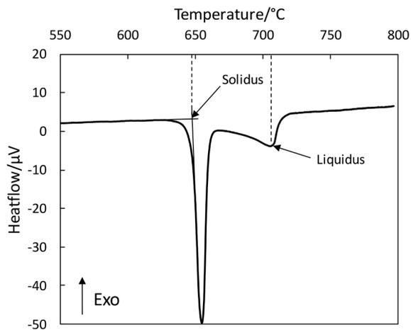
**Figure 1.** Classical DSC curve of a CaCl<sub>2</sub>-CaF<sub>2</sub> (70-30 mol.%) sample at 2 °C·min<sup>-1</sup>.
