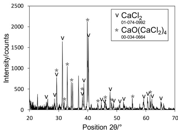
**Figure 5.** XRD pattern of CaCl<sub>2</sub>-CaO (87-13 mol.%) sample.
