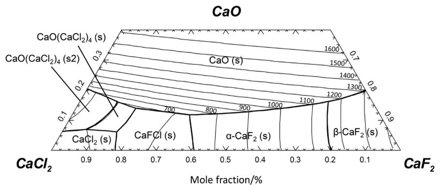
**Figure 7.** CaCl<sub>2</sub>-CaF<sub>2</sub>-CaO phase diagram calculated with FactSage®.
