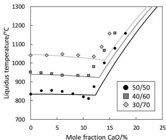
**Figure 8.** Liquidus cross-sections of the CaCl<sub>2</sub>-CaF<sub>2</sub>-CaO phase diagram (solid lines correspond to the model).
