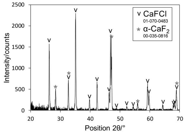
**Figure 3.** XRD pattern of CaCl<sub>2</sub>-CaF<sub>2</sub> (40-60 mol.%) sample.
