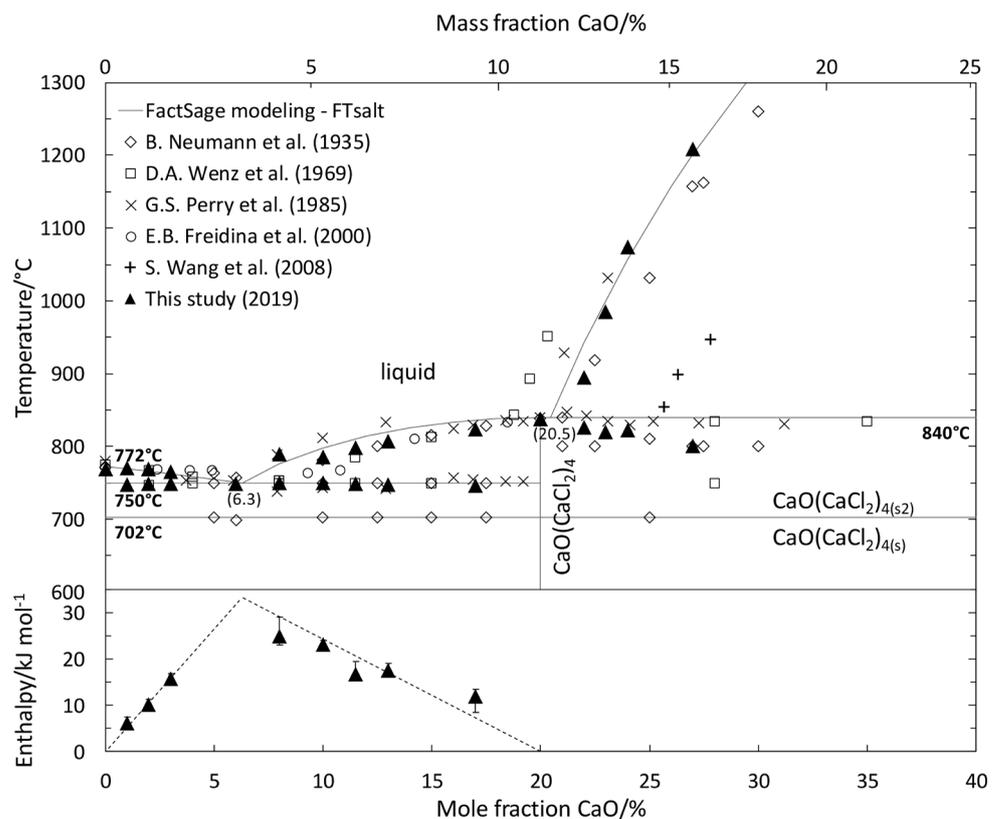
**Figure 4.** Phase diagram (upper part) and Tamman diagram (lower part) of the CaCl<sub>2</sub>-CaO system.
