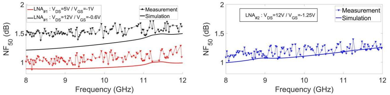
Fig. 6 : Simulated and measured X-band noise figure for LNA<sub>#1</sub> [in its **low noise configuration** ( $V_{DS}=5V / V_{GS}=-1V$ ), in **EM aggression mode** ( $V_{DS}=12V / V_{GS}=-0.6V$ )] and for LNA<sub>#2</sub> ( $V_{DS}=12V / V_{GS}=-1.25V$ )
