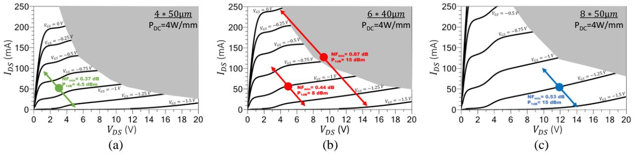
Fig. 2 : Static characteristics [ $I_{DS}(V_{DS})$ ] for three transistor dimensions ( $4*50\mu\text{m}$ ,  $6*40\mu\text{m}$  &  $8*50\mu\text{m}$ ). Each quiescent point appears with  $NF_{\min}$  and associated  $P_{1dB}$ . The areas of maximum DC power dissipation are shown in gray.
