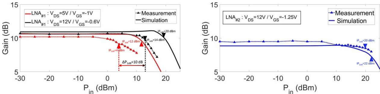
Fig. 5 : Simulated and measured gain vs. RF power at LNAs input for LNA<sub>#1</sub> [in its **low noise configuration** ( $V_{DS}=5V / V_{GS}=-1V$ ), in **EM aggression mode** ( $V_{DS}=12V / V_{GS}=-0.6V$ )] and for LNA<sub>#2</sub> ( $V_{DS}=12V / V_{GS}=-1.25V$ )
