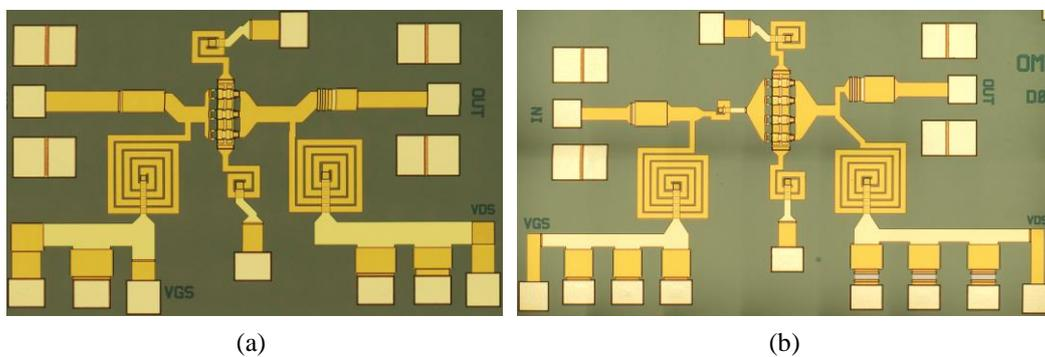
Fig. 3 : Layout of the two LNAs considered for the study: (a) LNA#1 with the  $6*40\mu\text{m}$  transistor, (b) LNA#2 with the  $8*50\mu\text{m}$  transistor.
