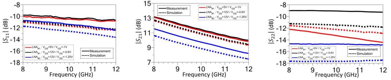
Fig. 4 : Simulated and measured S-parameters of LNA<sub>#1</sub> [in its **low noise configuration** ( $V_{DS}=5V / V_{GS}=-1V$ ), in **EM aggression mode** ( $V_{DS}=12V / V_{GS}=-0.6V$ )] and of LNA<sub>#2</sub> ( $V_{DS}=12V / V_{GS}=-1.25V$ )
