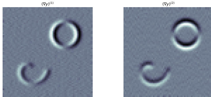
Fig. 2: The two components of the gradient \mathbf{y} = \nabla g , is the relevant quantity for the fidelity term of (CROC). Note that the noise on the image has an even greater impact on its gradient, such that a gradient denoising strategy must be adopted, especially for experimental images.
