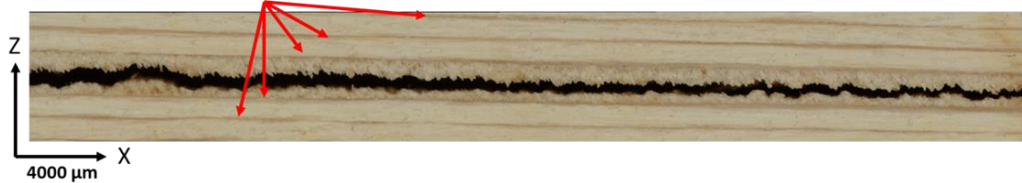
Figure 22 – Initiation and intra-ply migration (top) 90^\circ ply; intra-ply crack propagation in
