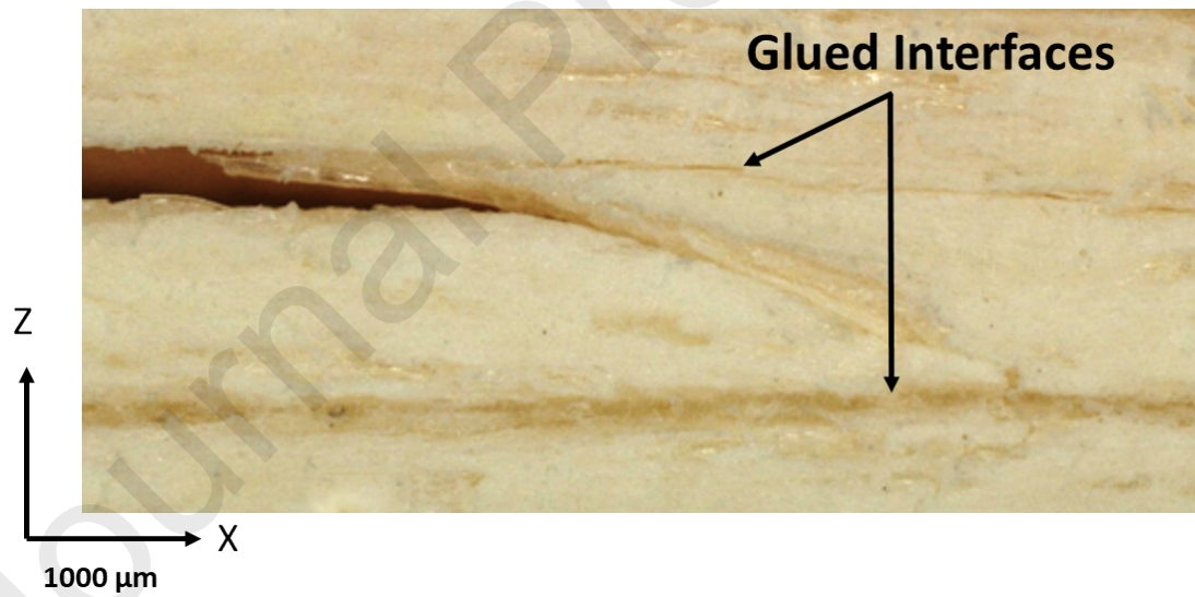
Figure 14 – Illustration of the crack path leaving the interfacial 0^\circ/0^\circ due to fiber out-of-plane angle
