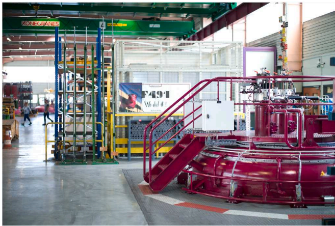
Fig. 6. Schematic representation and photograph of the top of industrial facilities for batch processing CVI [96,97].
