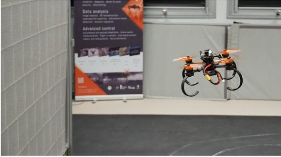
**Fig. 8** The quadrotor facing the wind indoor tunnel.
