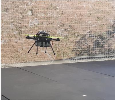
Fig. 2. The hexarotor flying in the Marseille's flying arena in front of the safety net. Through the safety net, we can see a textured panel considered here as a background wall
