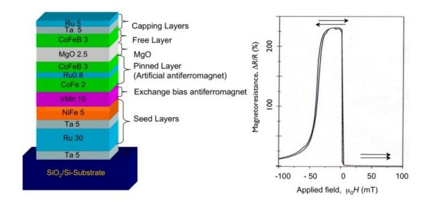
Figure 12 A thin film stack with a magnetic tunnel junction (left). The magnetic layer below the MgO tunnel barrier is pinned by coupling to the antiferromagnetic  $IrMn_3$  layer to produce the magnetoresistance characteristic (right).
