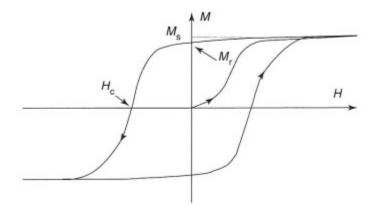
Figure 9 The hysteresis loop of M against H for a typical permanent magnet.  $M_s$  is the saturation magnetization,  $M_r$  the remanent magnetization at zero applied field, and  $H_c$  the coercive field required to reduce the magnetization to zero
