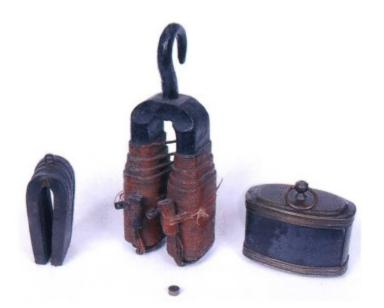
Figure 4 Magnets of four centuries shown clockwise from the left;  $18^{th}$  century horseshoe magnet;  $19^{th}$  century electromagnet;  $17^{th}$  century lodestone; and  $20^{th}$  century Nd<sub>2</sub>Fe<sub>14</sub>B
