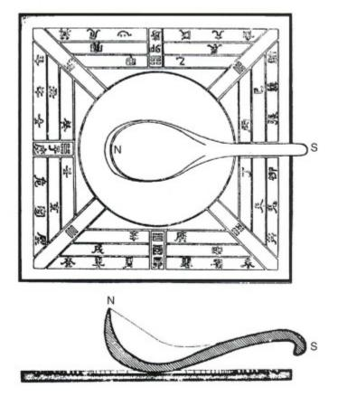
Figure 1 Baseplate and lodestone spoon of the South-pointer used in China from the first century B.C. (Needham 1962), courtesy of Cambridge University Press
