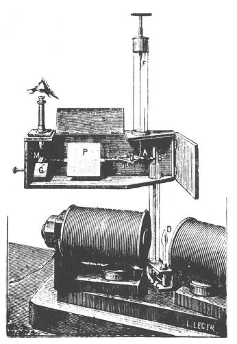
Figure 7 Pierre Curie's torsion balance used for quantitative measurements of magnetic susceptibility at high temperature in a horizontal magnetic field gradient (Curie 1895)
