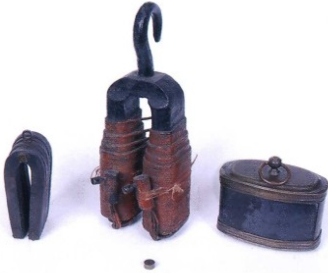
Figure 4 Magnets of four centuries shown clockwise from the left; 18 th century horseshoe magnet; 19 th century electromagnet; 17 th century lodestone; and 20 th century \text{Nd}_2\text{Fe}_{14}\text{B}
