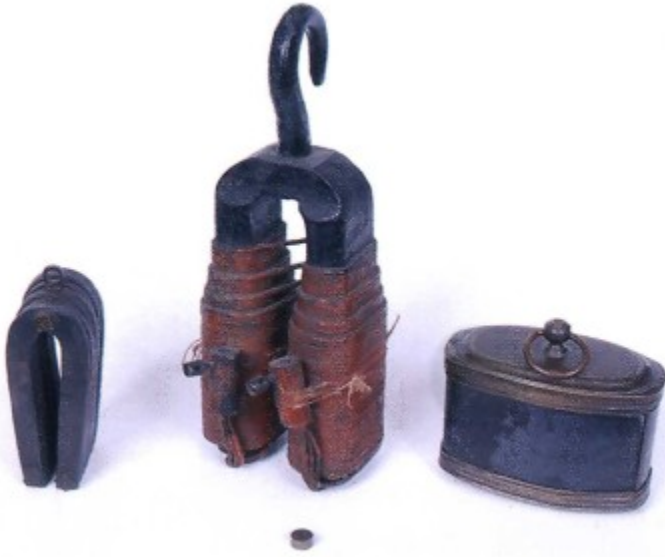
Figure 4 Magnets of four centuries shown clockwise from the left; 18 th century horseshoe magnet; 19 th century electromagnet; 17 th century lodestone; and 20 th century Nd 2 Fe 14 B
