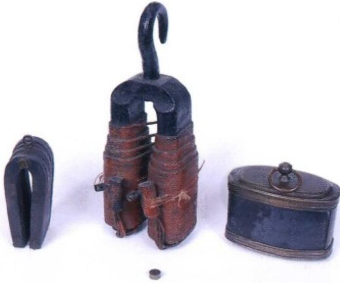
Figure 4 Magnets of four centuries shown clockwise from the left; 18<sup>th</sup> century horseshoe magnet; 19<sup>th</sup> century electromagnet; 17<sup>th</sup> century lodestone; and 20<sup>th</sup> century Nd<sub>2</sub>Fe<sub>14</sub>B
