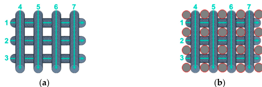
Figure 4. (a) Texturing process to generate micrometric square pillars; (b) texturing process to generate micrometric square pillars followed by irradiation of their tops.
