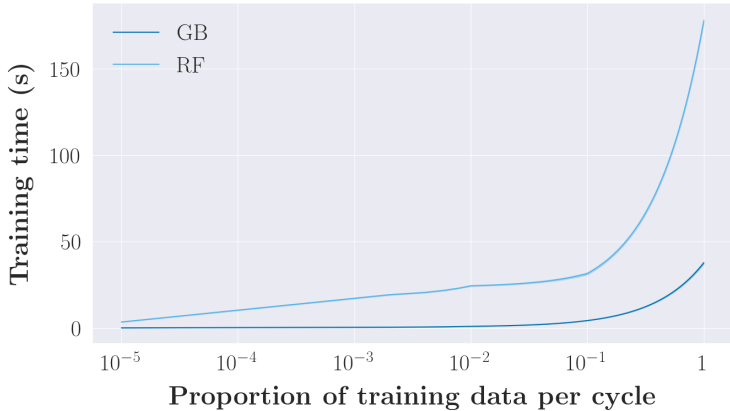
Figure 4: Training times of the optimized Gradient Boosted Trees (dark blue) and Random Forest (light blue) models for different training dataset sizes. The x-axis represents the proportion of training data selected from each dataset to form the final training dataset, while the y-axis represents the training time in seconds. Each curve depicts the average training time for a particular model, with a shadow indicating the standard deviation across 168 runs.
