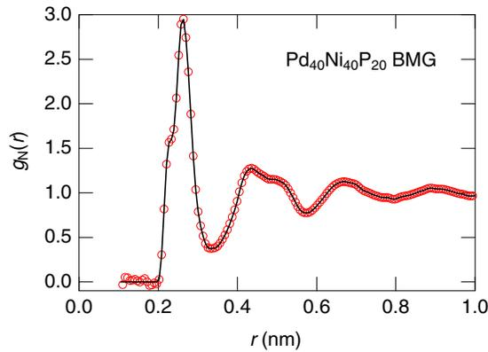
FIG. 2. Circles represent experimental  $g_N$  data and the solid curve shows the corresponding fit from RMC modeling.
