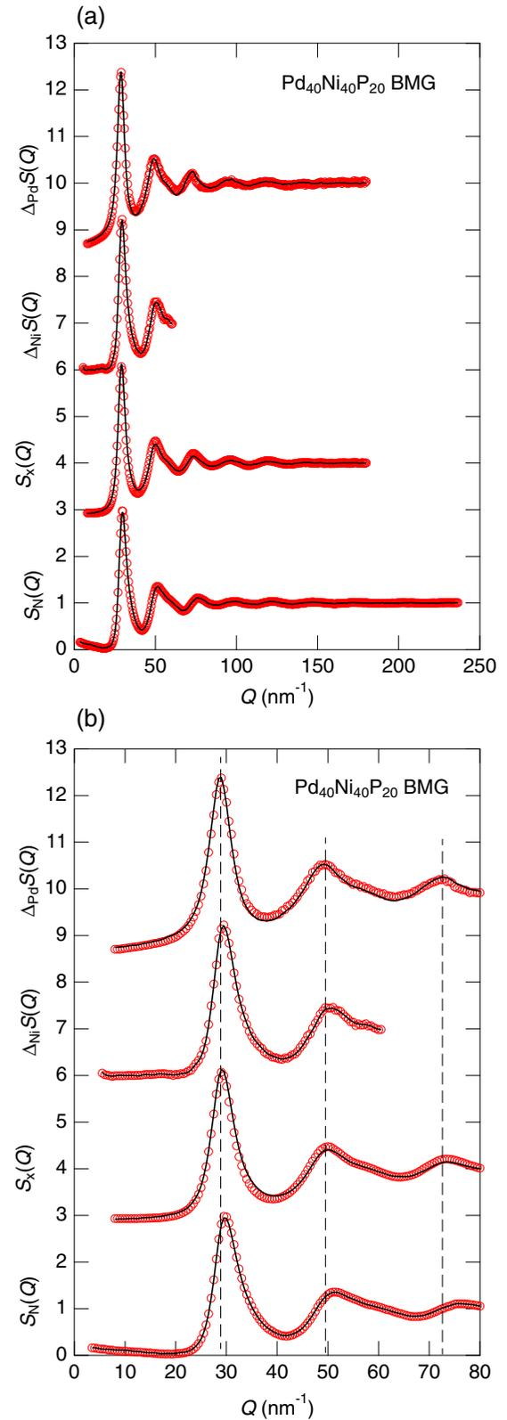
FIG. 1. From top to bottom, circles denote experimental data of  $\Delta_{\text{Pd}}S(Q)$  and  $\Delta_{\text{Ni}}S(Q)$  taken from AXS, and  $S(Q)$ s by XD and ND in the (a) whole  $Q$  range measured and (b) in the low- $Q$  range up to 80 nm<sup>-1</sup>. Solid curves show the corresponding fits from RMC modeling. For clarity, the spectra are displaced upward by 3.
