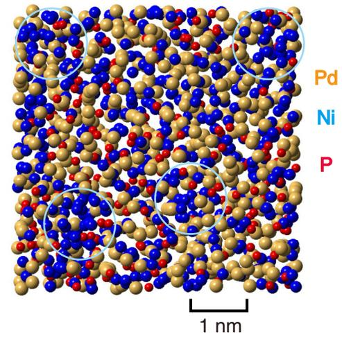
FIG. 6. Three-dimensional atomic representation obtained from the RMC calculation. The circles indicate the Ni-rich regions, and their diameter of 1.26 nm corresponds to a  $Q$  value of  $5 \text{ nm}^{-1}$ .
