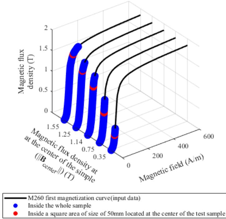
Figure 3: Distribution of  $\mathbf{H}$  and  $\mathbf{B}$  inside different areas of the test sample for several values of  $\|\mathbf{B}_{\text{center}}\|$  and with  $T_y = 200$  mm. *Source: authors own work*
