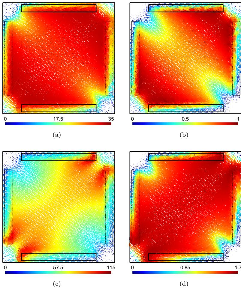
Figure 2: Distribution of  $\mathbf{H}$  (left) and  $\mathbf{B}$  (right) inside the test sample for  $\|\mathbf{B}_{\text{center}}\| = 0.75 \text{ T}$  (top) and  $\|\mathbf{B}_{\text{center}}\| = 1.55 \text{ T}$  (bottom). *Source: authors own work*
