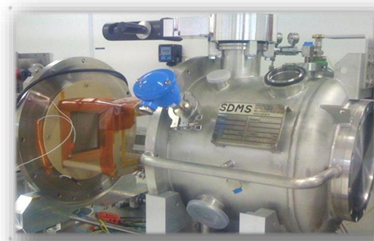
View of the detection part ( anode and detection cage) on a picture of the \mu TPC( opened)
